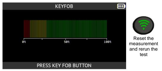
The tool will wait for a signal and then display the strength of the signal it receives.
