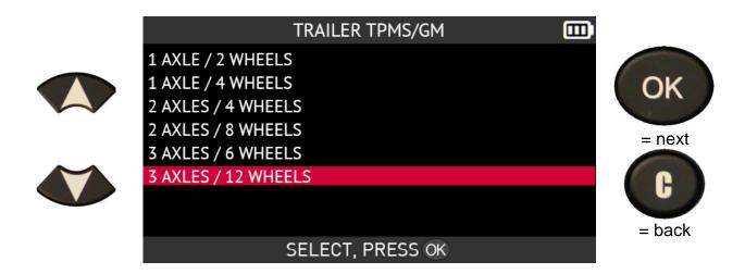
Place the tool close to the sidewall of the **left front** tire of the trailer at the level of the **left front** wheel valve and then press the **Read sensor** button to come out of standby and read the sensor.
