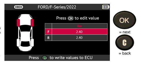
Use the up arrow button to increase the reference pressure value of the selected wheels and the down arrow button to decrease the value.
