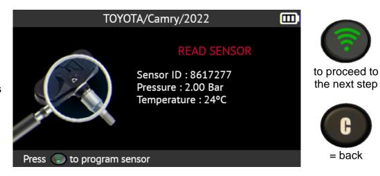
Position the new sensor in above the tool's antenna to carry out the programming.
