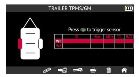
When you choose to check the sensors of a trailer with 12 wheels, the icon bar is not displayed at the bottom of the screen.
