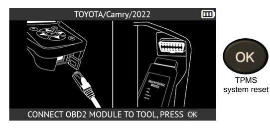
When the vehicle's TPMS system has been reset, the tool will return to the TPMS service screen.
